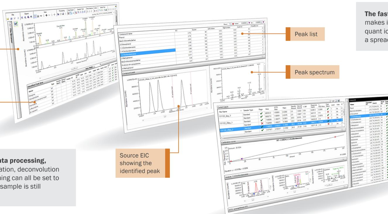
The fast qual-to-quant workflow in TOF-DS makes it easy to import target compounds, quant ions and retention time windows from a spreadsheet.
