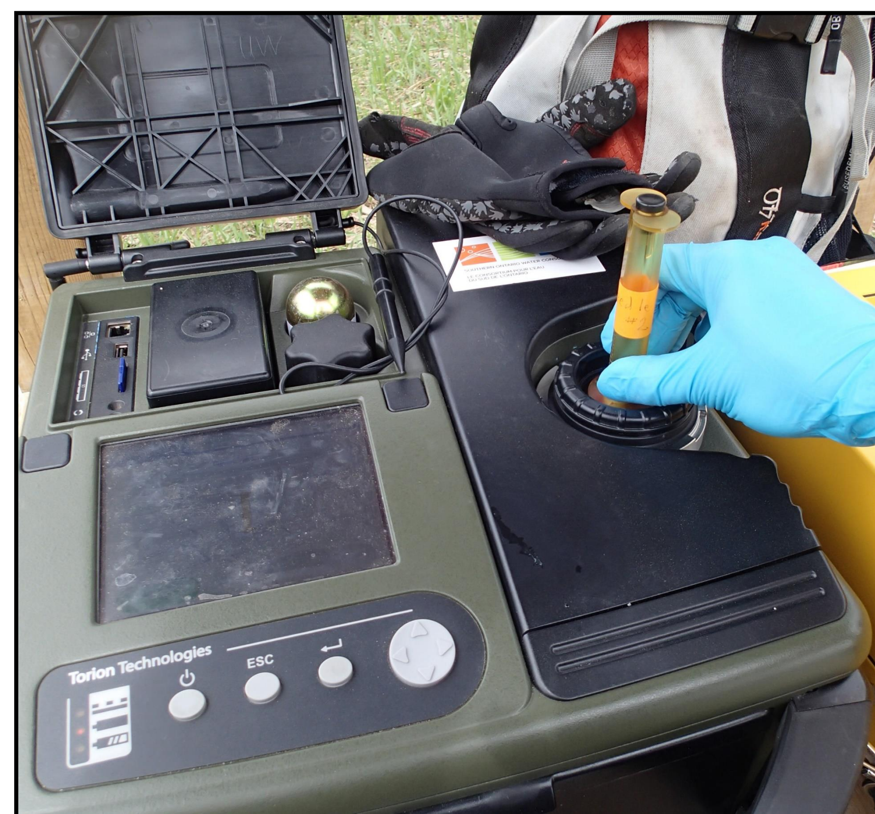
Step 4: desorption of NTD into instrument for analysis
