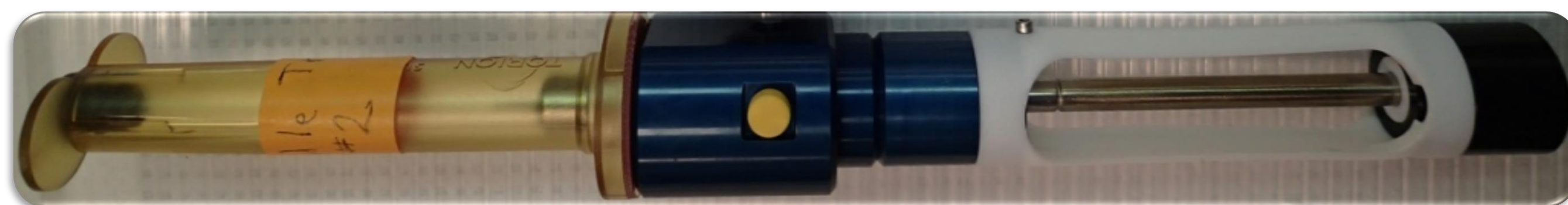
Step 2: needle trap device (NTD) is linked with the conventional trap holder such that analyte will be transferred from the TFME membrane to the NTD once inserted into the SPS-3 high volume desorption unit
